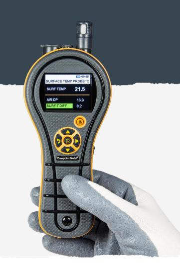
The steel surface temperature generally should be at least 3°C above the dew point when paints are applied. Below this temperature the Dewpoint Meter will sound an alarm and the display colour will change to warn you that the surface conditions are not suitable too paint.
