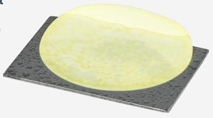
The test involves the reaction of soluble ferrous iron salts with potassium ferricyanide to form ferric hexacyanoferrate, which is commonly known as prussian blue. The relatively high tinting strength of prussian blue enables the reaction to be used as a very sensitive test on ferrous irons.
