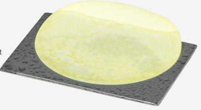
If soluble salts remain, these will be drawn by capillary action into the Potassium Ferricyanide Paper and will react and give a prussian blue dot effect on the Potassium Ferricyanide Paper corresponding to the contaminated pits on the blast-cleaned steel.
