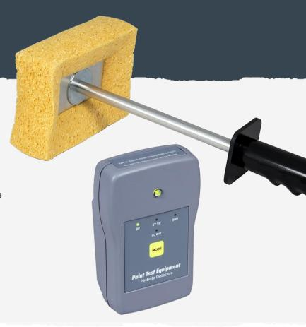
Operation is by a wet sponge, moistened with a wetting agent, being moved over the coating. The wetting agent penetrates any pinhole and makes a conductive path through to the substrate.
