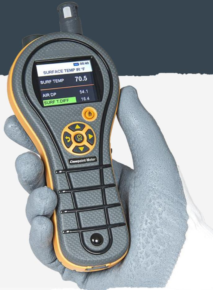
The steel surface temperature generally should be at least 3°C above the dew point when paints are applied. Below this temperature the Dewpoint Meter will sound an alarm and the display colour will change to warn you that the surface conditions are not suitable to paint.
