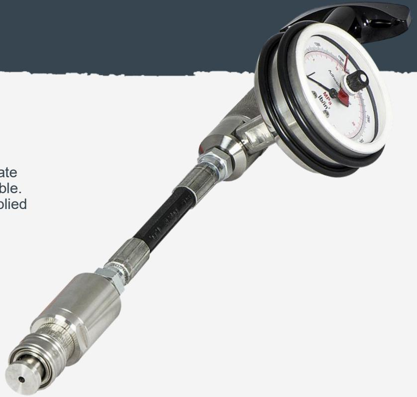
The adhesion is measured by the tensile pull on a Dolly glued to the coating surface. The force is applied through the centre of the Dolly by a hydraulically loaded pin. This ensures an exactly central point-loading of the force.
